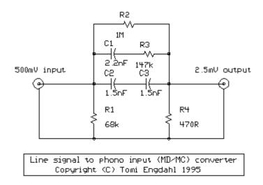
This circuit is a simplified version of circuit published in Elektor Electronics (T.Giesberts, Pickup input becomes line input, Elektor Electronics, December 1995, page 99). The basic circuit idea is same, but my circuit is simpler and it does not use high-precision components. The performance is not the same, but I think that this circuit build even from 5% components is adequate for many purposes.
